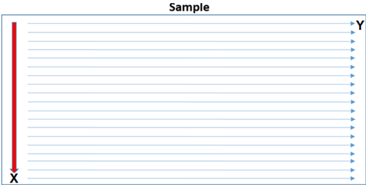
Figure 2.6 Raster scan, Y (slow signal), X (fast signal)
