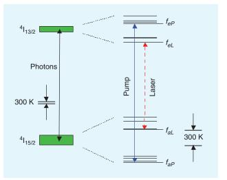
Figure 2.  $Er^{3+}$  ground state manifold and first excited state manifold. The scale on the right is magnified.
