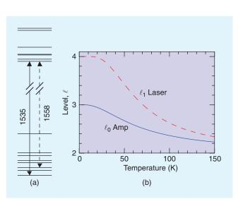
Figure 4.  $Er:Sc_2O_3$ ,  $\lambda_p = 1535 \text{ nm}$ ,  $\lambda_L = 1558 \text{ nm}$ : (a) energy levels, pump and laser transitions, (b) temperature dependence of the level parameters.
