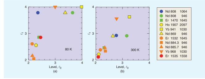
Figure 7.  $\ell_1$  vs  $\ell_0$  for a variety of known lasers at (a) 80 K and (b) 300 K. The color is keyed to the quantum defect. The host material is YAG in all cases, except in the last case, where the host is  $Sc_2O_3$ .
