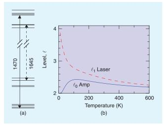
Figure 3. Er:YAG,  $\lambda_p = 1470 \text{ nm}$ ,  $\lambda_L = 1645 \text{ nm}$ : (a) energy levels, pump transition (solid line), and laser transition (dashed line), (b) temperature dependence of the level parameters.
