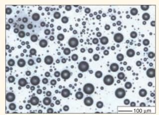
Figure 3. Optical spectroscopy experiments performed on water microdroplets that are standing on a superbydrophobic surface at Koç University (Courtesy: A. Kiraz Lab).
