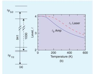
Figure 6. Yb:YAG,  $\lambda_p = 941 \text{ nm}$ ,  $\lambda_L = 1030 \text{ nm}$ : (a) energy levels, pump and laser transitions, (b) temperature dependence of the level parameters.
