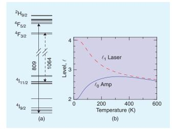
Figure 5. Nd:YAG,  $\lambda_p = 809 \text{ nm}$ ,  $\lambda_L = 1064.1 \text{ nm}$ : (a) energy levels, pump and laser transitions, (b) temperature dependence of the level parameters.
