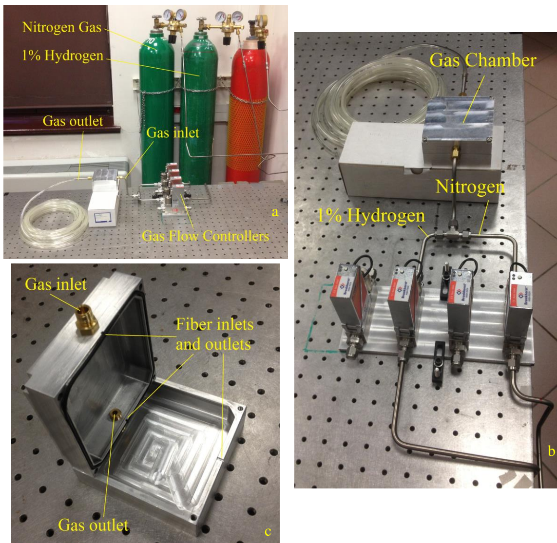
Figure 5.7 Gas sensing experiment setup. a) General view of the setup. b) Closer view of gas flow controllers. c) Closer view of the gas chamber.
