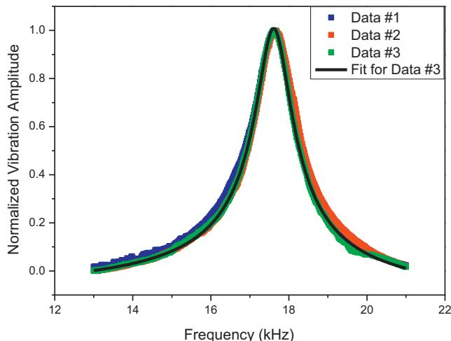
**Fig. 4.** An example of experimentally measured cantilever frequency response. The three shown sets of data correspond to three consecutive measurements carried out with a 200  $\mu\text{m}$ -long cantilever in gaseous CO<sub>2</sub> at 298 K and 5.63 MPa.
