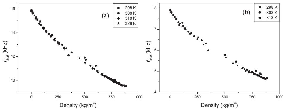
**Fig. 9.** Variation of  $f_{\text{fluid}}$  with density for (a) 225 \$\mu\text{m}\$ cantilevers and for (b) 325 \$\mu\text{m}\$ cantilevers.
