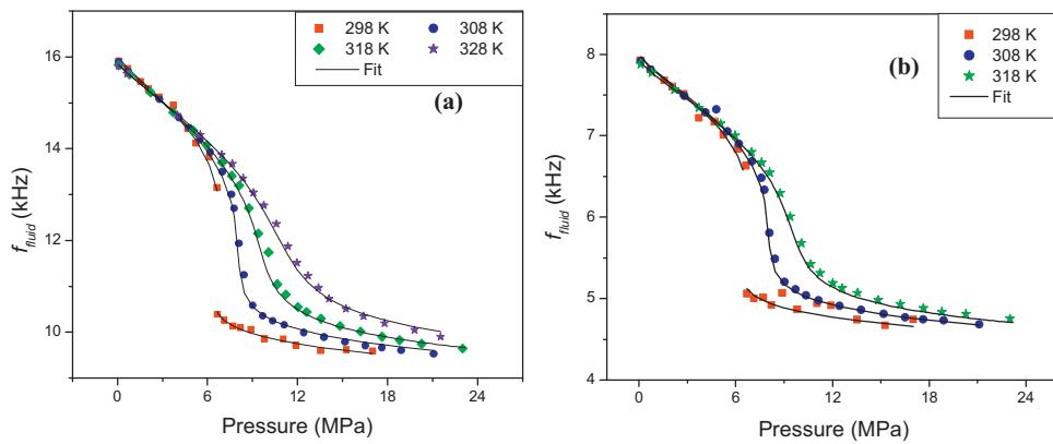
**Fig. 10.** Comparison of the experimental values of  $f_{\text{fluid}}$  (symbols) to the model of oscillations of a hydrodynamically damped cantilever (Eq. (7); solid lines) for (a) 225  $\mu\text{m}$  and (b) 325  $\mu\text{m}$  cantilevers at different  $\text{CO}_2$  temperatures.
