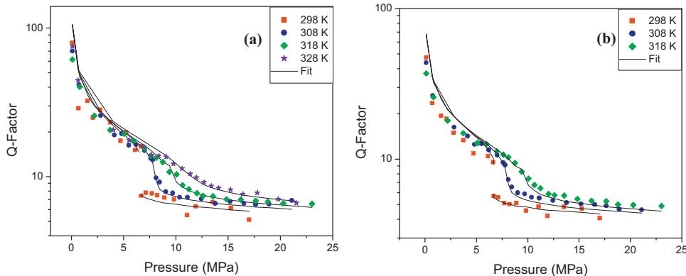
Fig. 12. Comparison of the experimental values of Q-factor (symbols) to the model of oscillations of a hydrodynamically damped cantilever (Eq. (8); solid lines) for (a) 225  $\mu\text{m}$  and (b) 325  $\mu\text{m}$  cantilevers at different  $\text{CO}_2$  temperatures.
