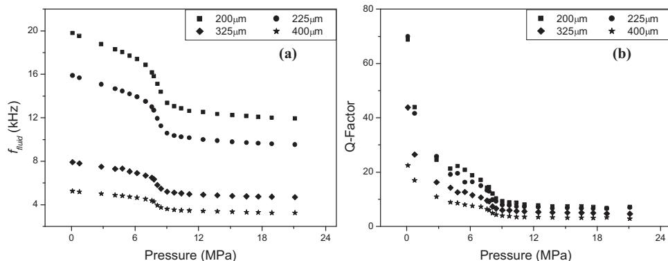
**Fig. 6.** Variation of (a)  $f_{fluid}$  and (b) Q-factor with pressure at 308 K for different cantilever lengths.
