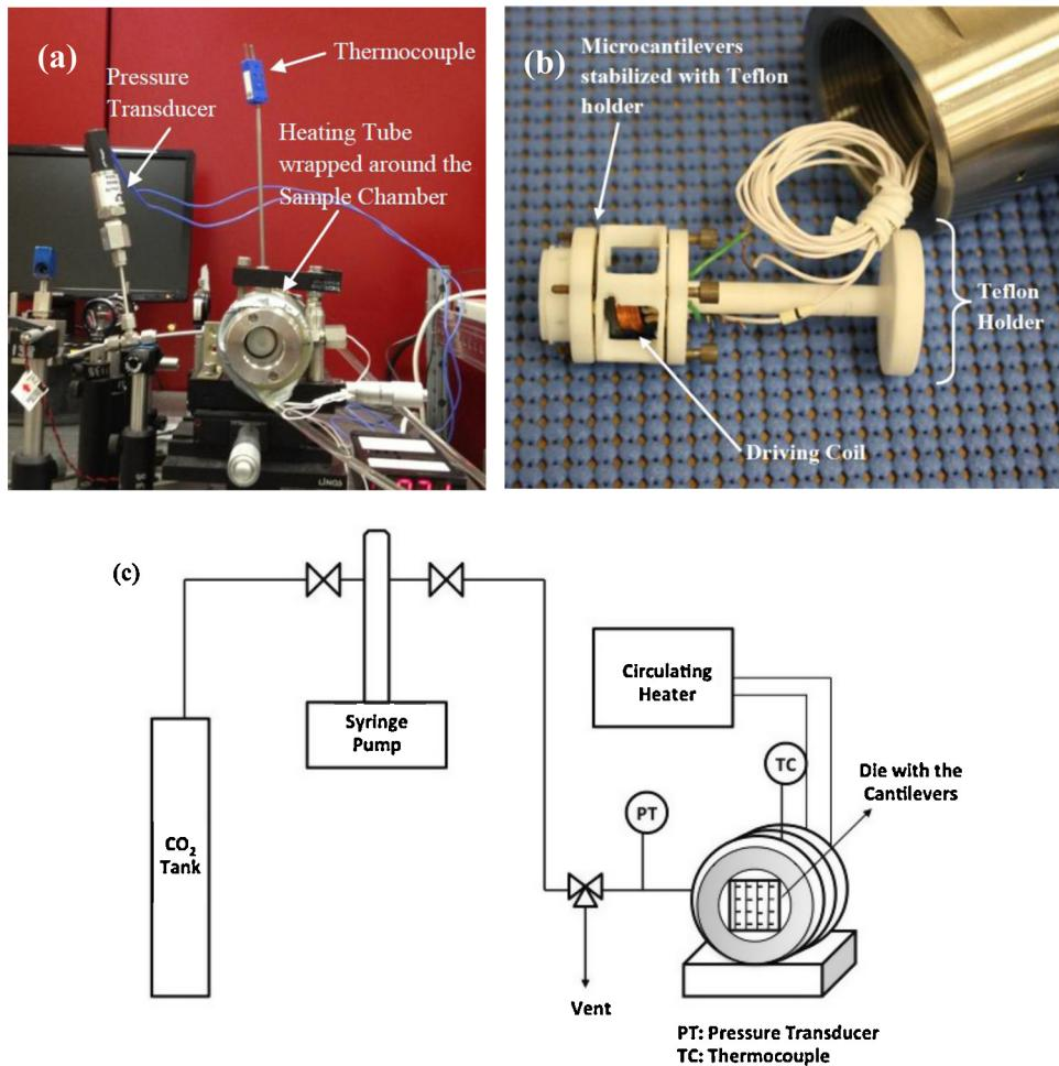
**Fig. 3.** (a) High-pressure sample chamber mounted on an  $x$ - $y$ - $z$  translation stage with attached pressure transducer, thermocouple, and heating tubing. (b) Detail of Teflon holder bearing the die with microcantilevers and the driving coil. (c) Schematics of the system for the sample chamber pressurization.
