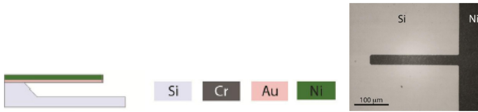
Fig. 1. (left) Schematic representation of microcantilever used for the fluid density and viscosity measurements (right) micrograph of the microcantilever.
