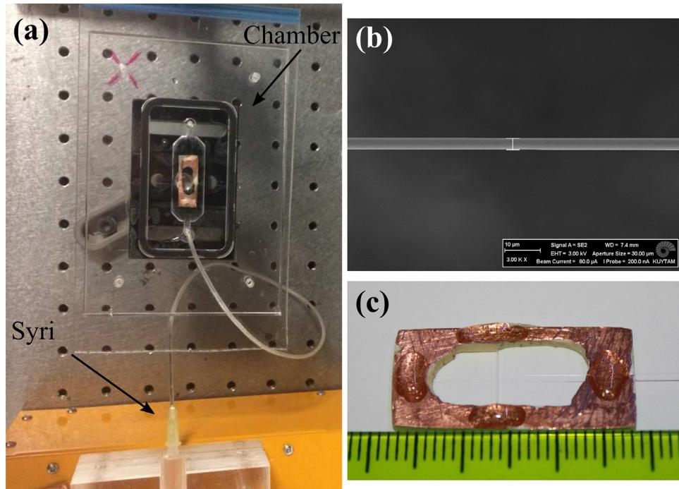
**Fig. 2.** (a) Picture of the sample chamber with the detector and the syringe pump. (b) An SEM image of a tapered fiber. Scale bar is 10  $\mu\text{m}$ . The thickness at the thinnest portion of the tapered fiber is measured to be  $\sim 3.2 \mu\text{m}$ . (c) Holder for the OFR and tapered fiber. Scale increases by 1 mm.
