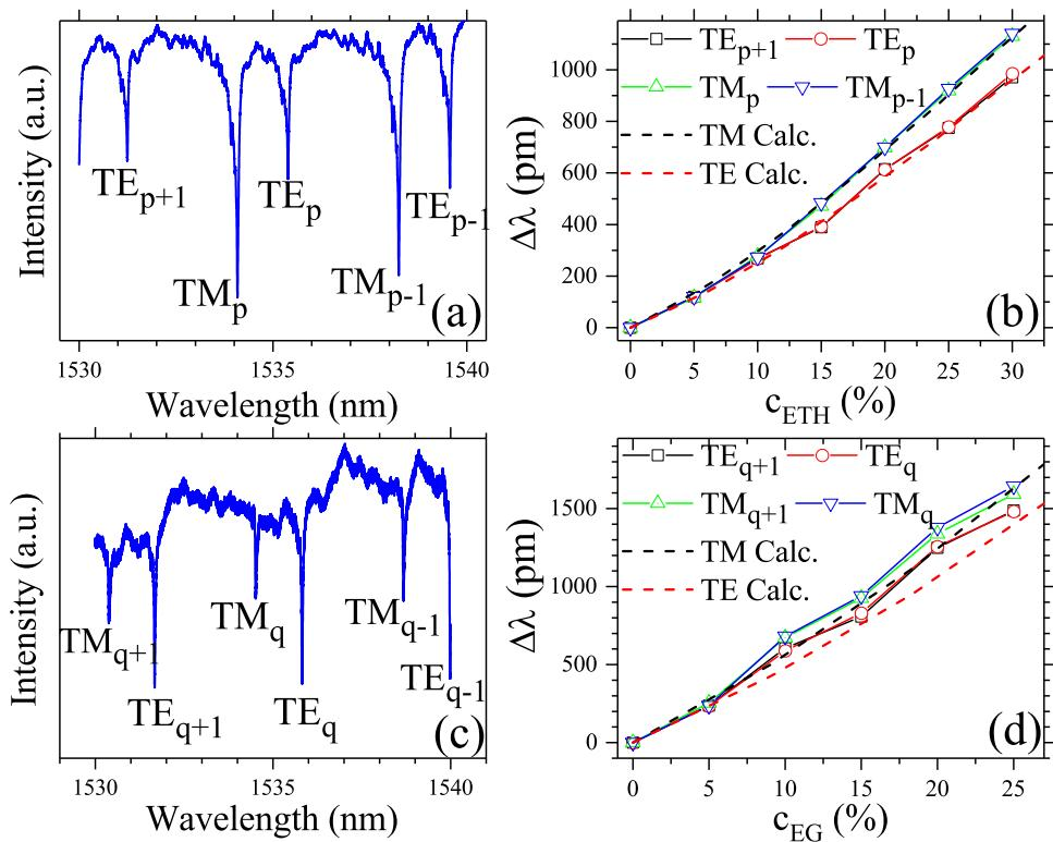
**Fig. 4.** Exemplary transmission spectra recorded during experiments using water solutions of (a) ethanol and (c) EG. From the WGMs depicted in the transmission spectra, four were selected for analysis under changing concentrations of ethanol or EG. Respective spectral shifts of the WGMs are depicted in (b) and (d) together with the theoretical predictions for TE and TM polarizations shown by dashed lines.
