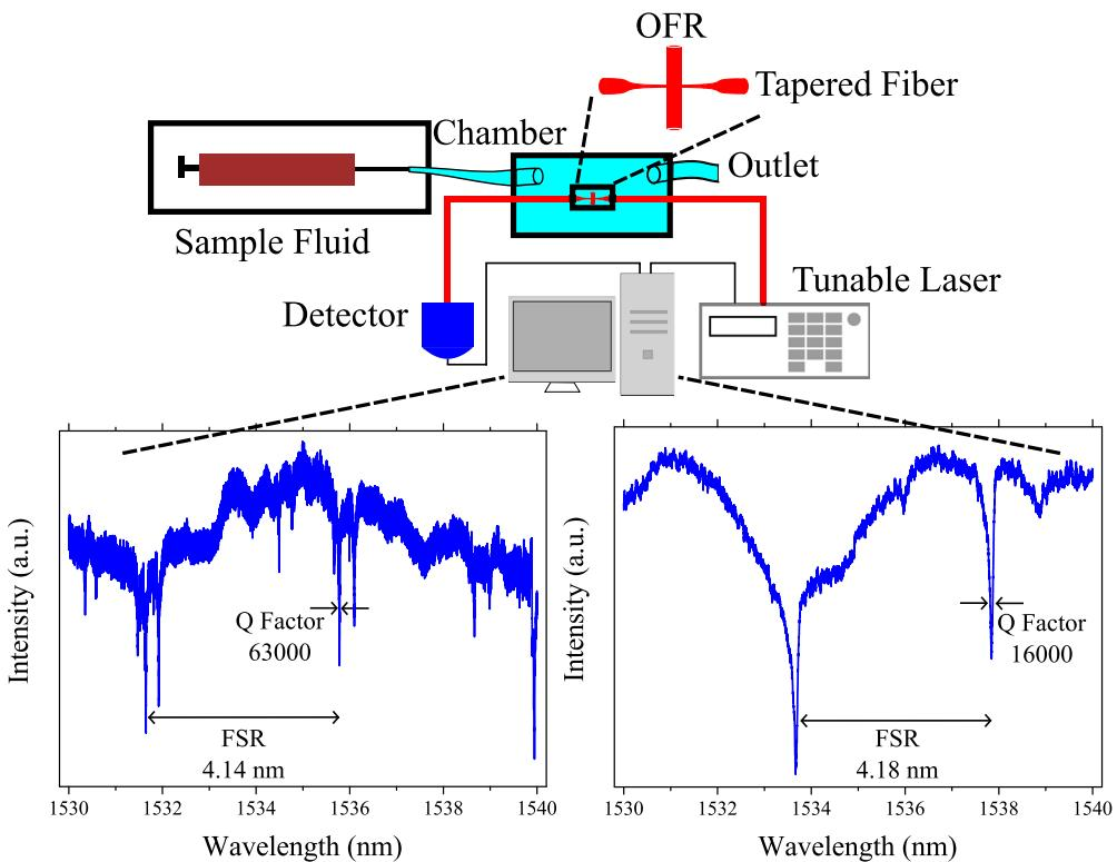
**Fig. 1.** (a) Schematic description of the fiber tapering and sensor characterization setups used in the experiments. Exemplary transmission spectra recorded from a sensor device while the chamber is filled with (b) air (Q-factor: 63000, FSR: 4.14 nm) and (c) water (Q-factor: 13000, FSR: 4.18 nm) are shown.
