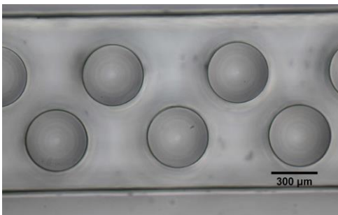
Fig 2.2. Microfluidic Channel with \mu pillar diameter of 300 \mu m using Al mold.
